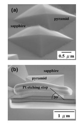
Fig. 2. (a) Tilted SEM view of the pyramids; (b) FIB cross-sectional image of a pyramid.
