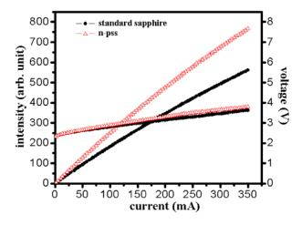
**Fig. 4.** (Color online) L-I-V curves of LED chips on the n-pss wafer and the standard sapphire wafer.
