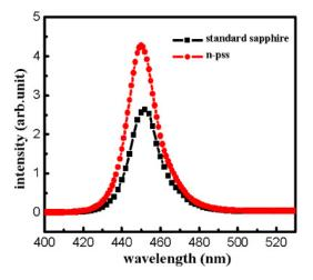
**Fig. 3.** (Color online) PL measurements of the GaN epilayer grown on the n-pss wafer and the standard *c*-plane sapphire wafer.
