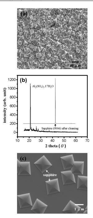
Fig. 1. (a) Etching-product layer on the etched sapphire surface; (b) diffraction pattern of the  $Al_2(SO_4)_3 \cdot 17H_2O$  phase; (c) enlarged SEM image of the facet pyramids on the n-pss wafer surface.
